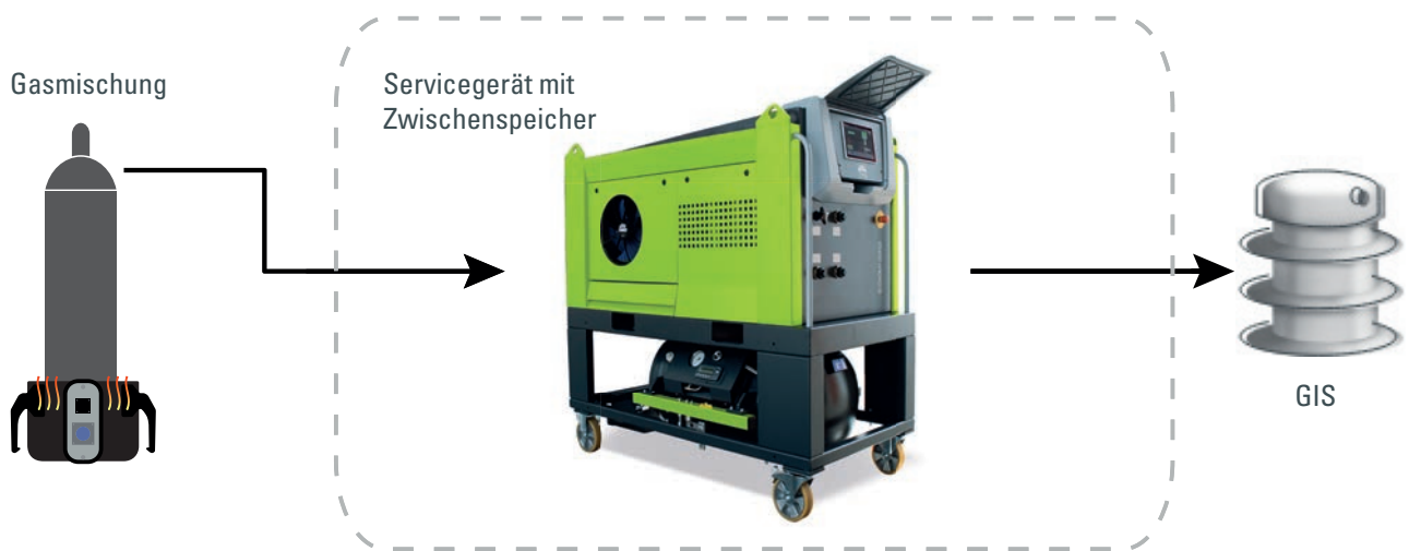
Figure 3: Illustration of the operating principle of a service cart with integrated buffer tank for the removal of partially liquefied mixtures from a heated pressure vessel.
